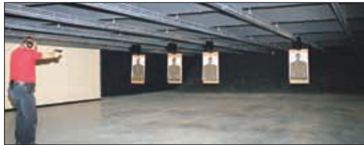
Sergeant Gregory Otto uses one of the three pistol firing ranges. The unique ventilation system completely exchanges the air every 87 seconds and provides a negative pressure so no air escapes from the room. The back wall contains several feet of shredded used tires to stop bullets.
