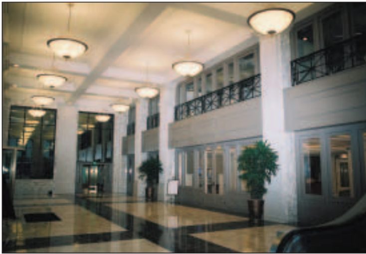
The PrivateBank's impressive lobby combines original marble with reconditioned features and period design lighting to maintain the historical look. The lights, from Visa Lighting, were hand-painted by a local artist to resemble the alabaster lights in the offices. They're equipped with compact fluorescent lamps.
