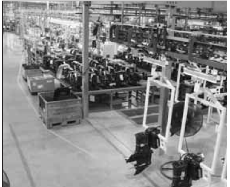
Renovating the Bombardier facility was the second time around for Roman Electric, which designed and built the huge, original electrical system for Golden Books. Here, outboard engines near completion on Bombardier’s powerhead assembly line.
