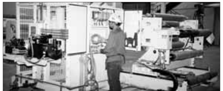
Control wiring for an unwinder on the process line is installed by Roman electrician Jason Schuebel.
